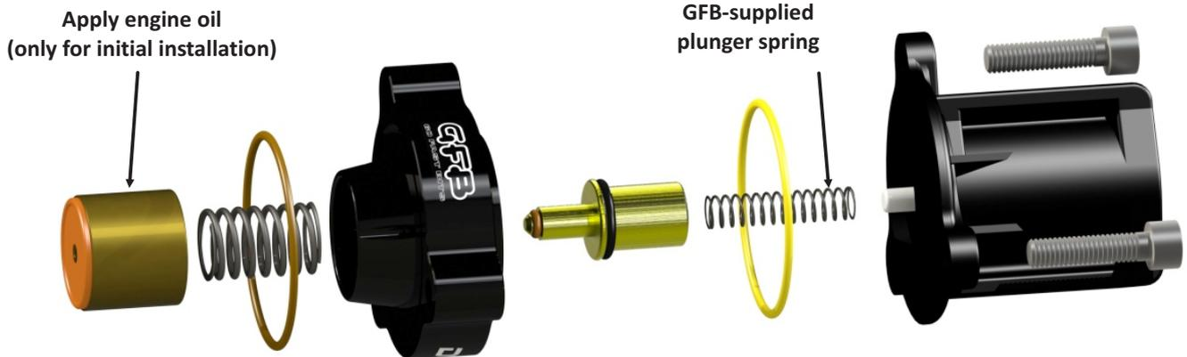
During assembly, check that the piston slides freely in the body without sticking or binding. It is a very close fit and can sometimes be difficult to get started into the bore, but once in it should move without needing to be forced.
